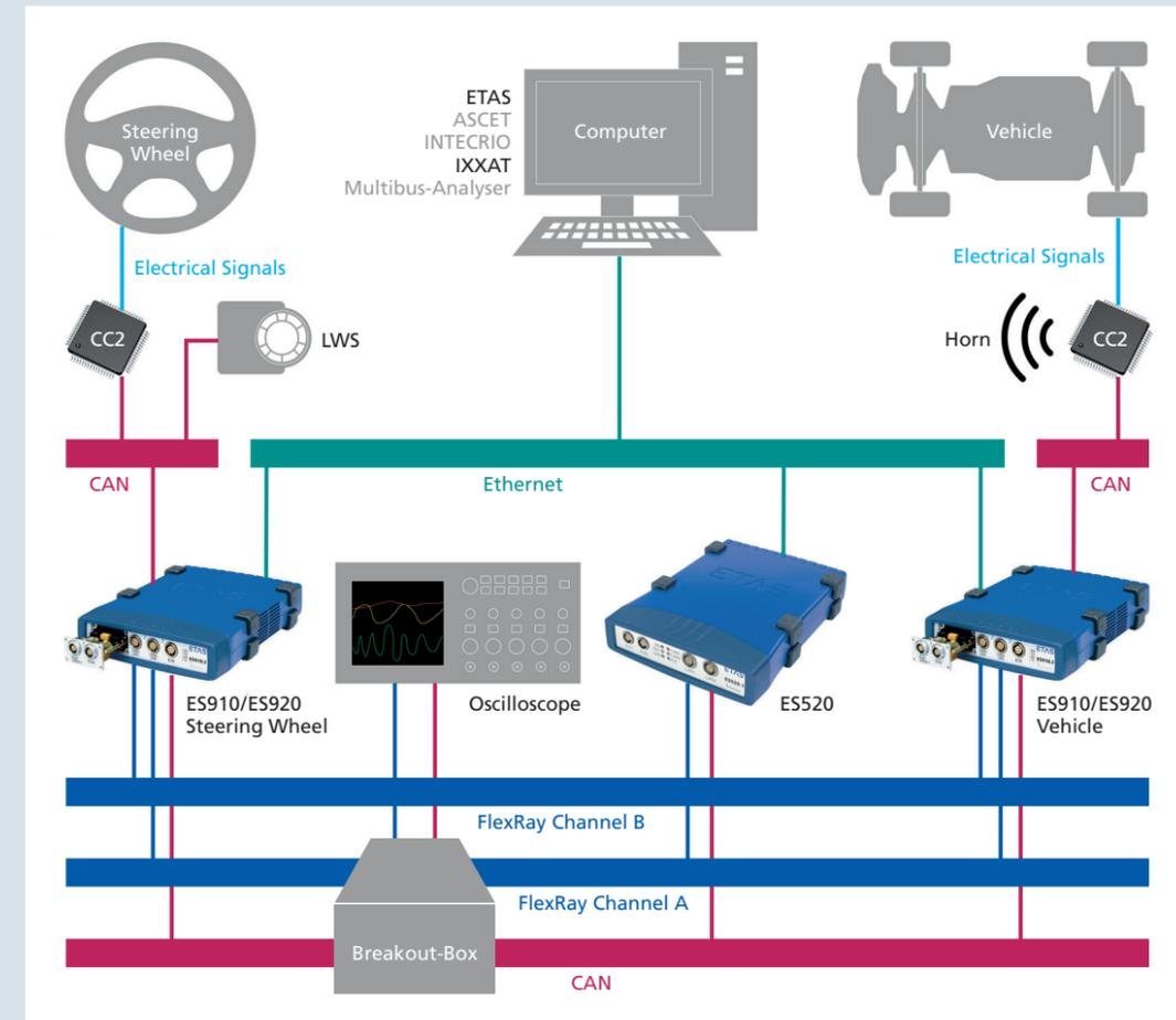
Schematic layout of the test bench
