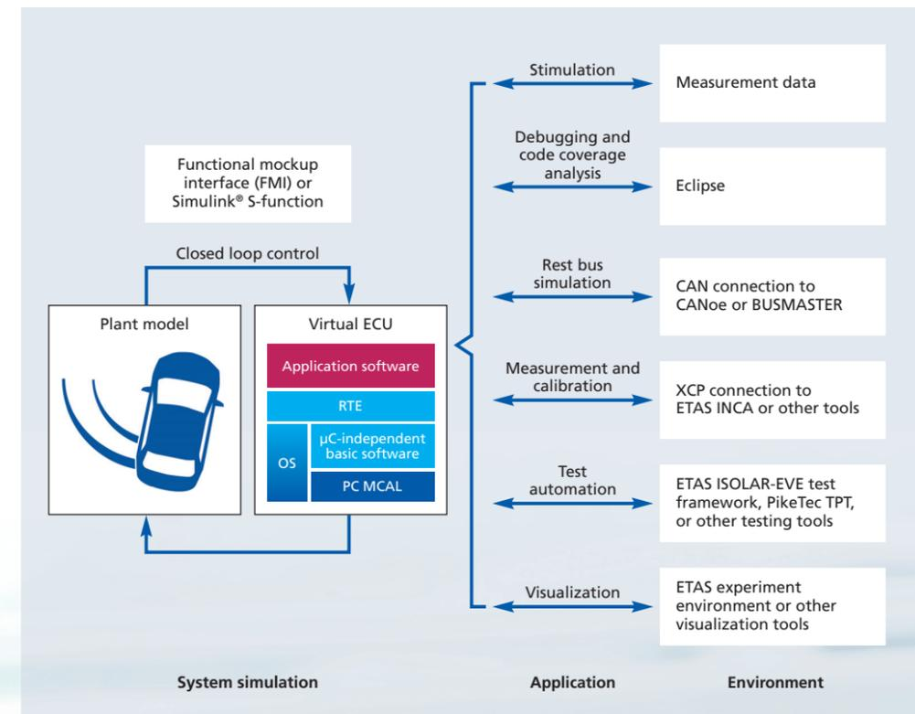
The openness of ISOLAR-EVE enables flexible integration into available tool environments.
