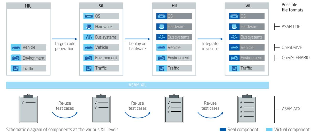
Schematic diagram of components at the various XiL levels
