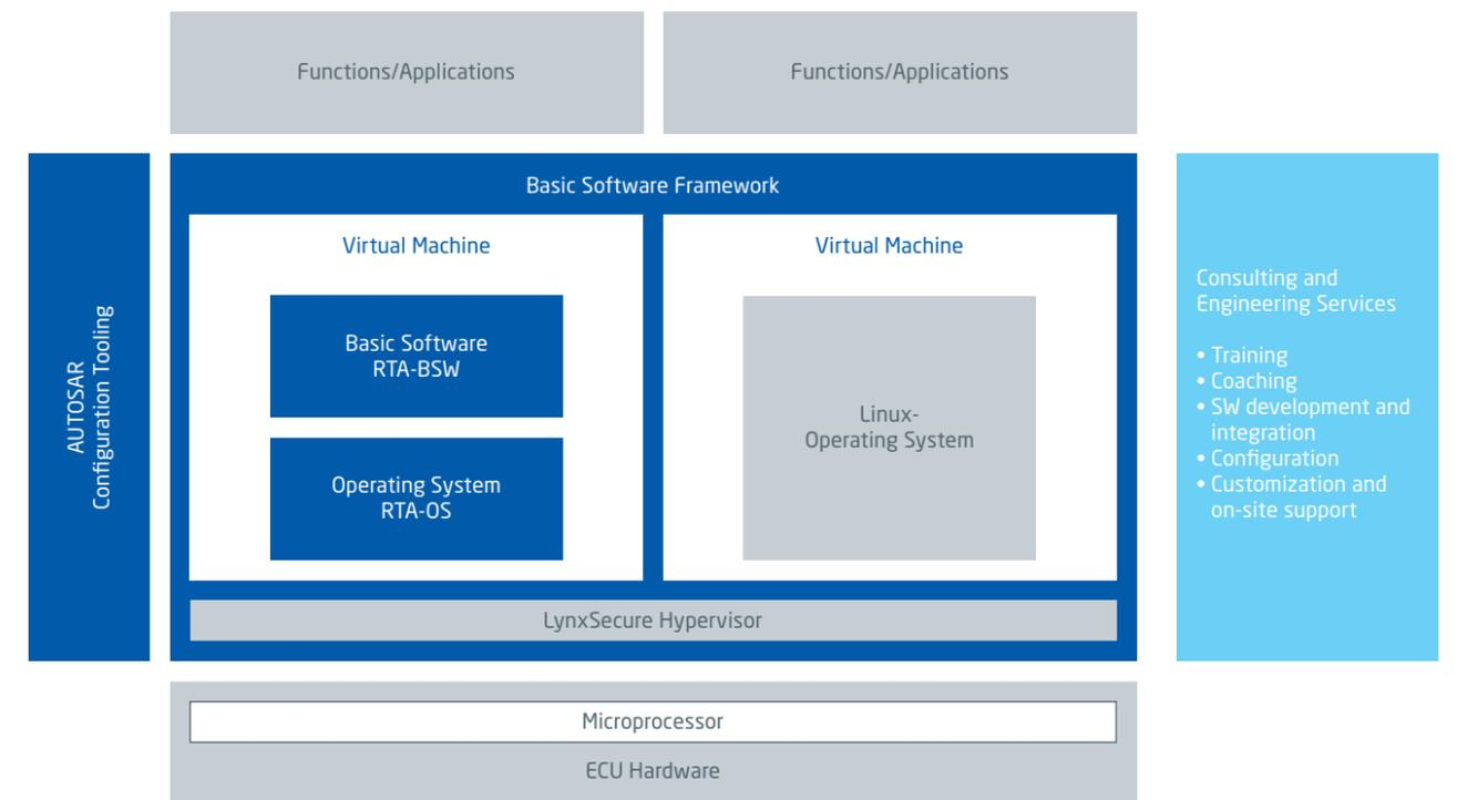
Dividing the processor cores into separate virtual machines makes it possible to manage the complexity of the software
