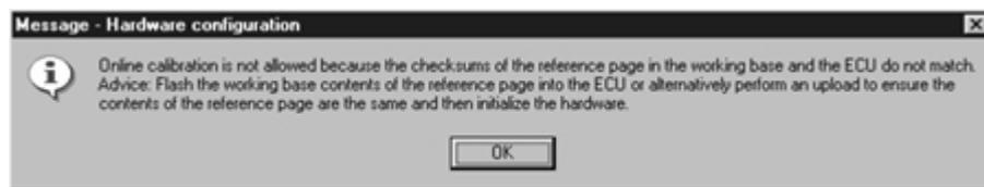
Fig. 2-1: Error message in case of a reference page mismatch
