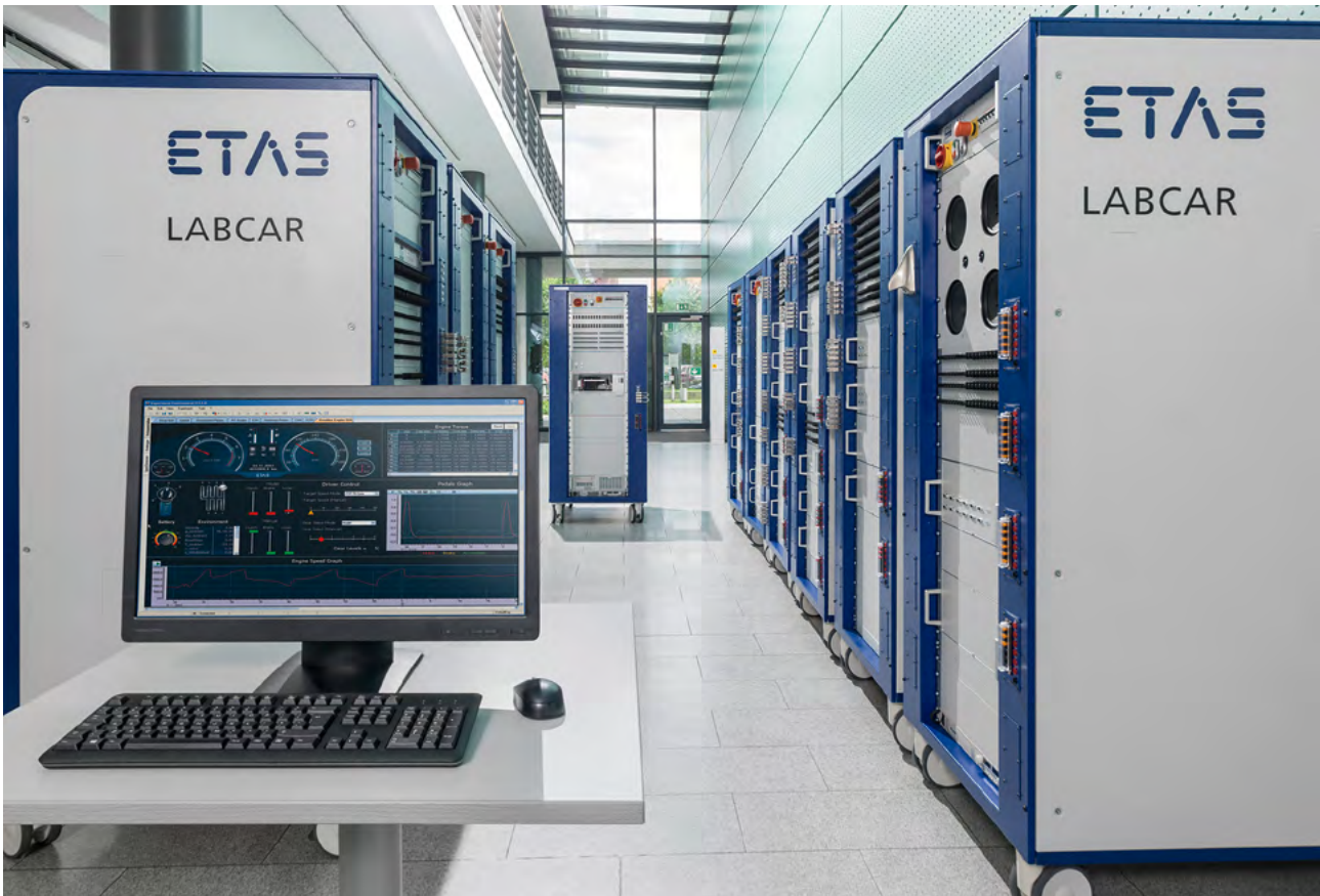
Fig. 2: HiL test bench for ETAS NETWORK-LABCAR.
