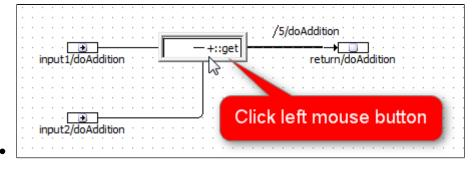
4. Result: return block input pin is connected to output pin of "+" operator
